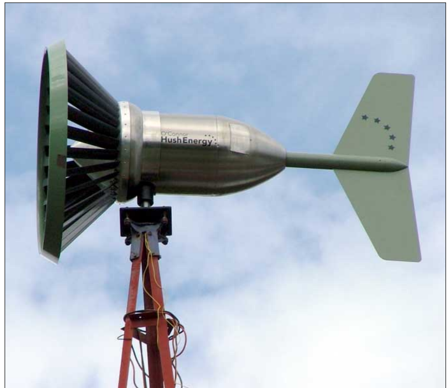
The Hush turbine newly installed on the tower at CERES, before the wiring was complete.
